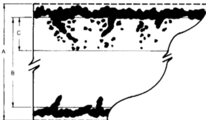
$$\text{Metal Loss (mils/side)} \left[ \left( \frac{A-B}{2} \right) \right]$$
