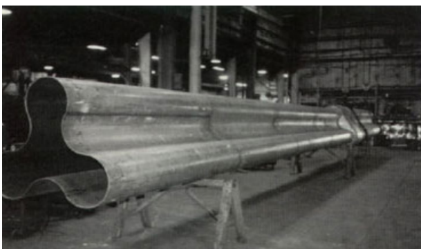
Large Welded retort fabricated from 0.375 inch (9.5 mm) HR-160® plate.
