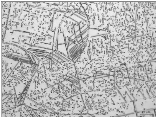
Microstructure of Mill Annealed G-35 ® Sheet After Aging for 8000 h at 760°C (1400°F)
